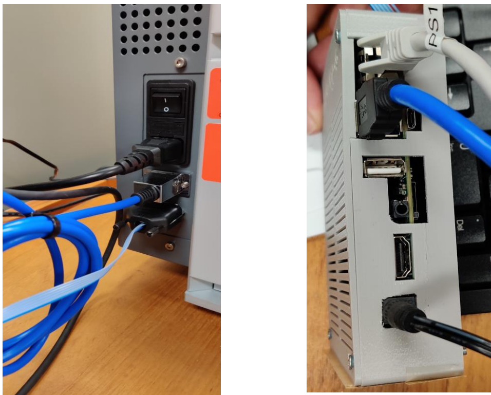
Figure 33: (left) Placement of canbus and firewire cable at back of instrument. (right) Placement of USB 3.0 and firewire cable at back of the Linux board
