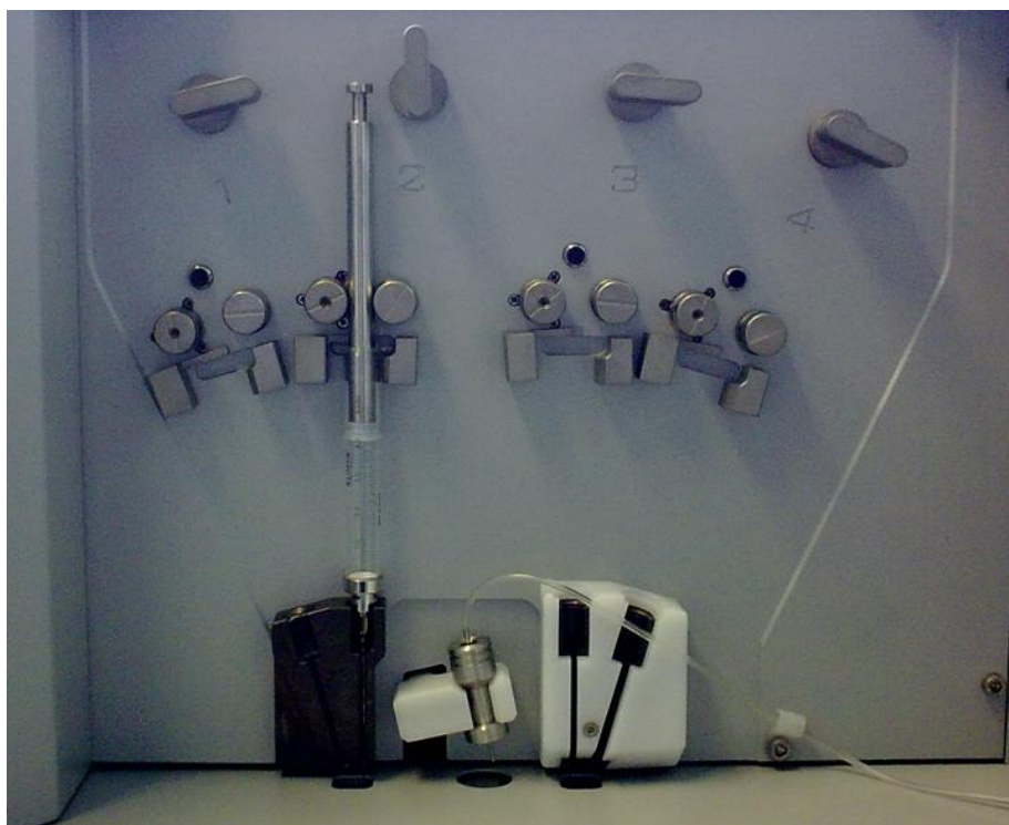
Figure 9: Inside door of the PamStation®12 and placement of a syringe.
